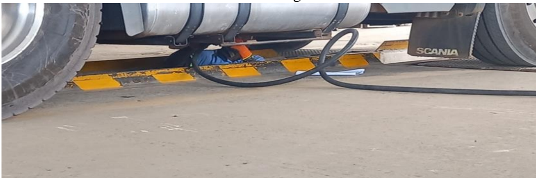
Figure 2: Securing emission test probe into exhaust pipe of a vehicle at NIT Vehicle Inspection Centre
